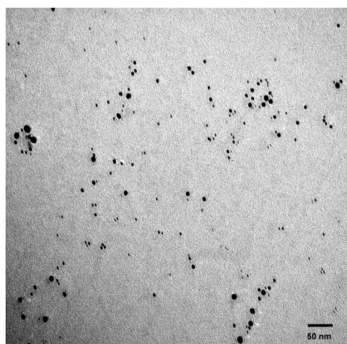
**Figure (2): Transmission Electron Microscope (TEM) micrographs of the biosynthesized AgNPs obtained from *F. solani* (scale bar equivalent to 50 nm).**
